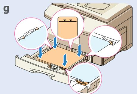
Ensure that the paper corners are under the corner snubbers. Do not fill above this line.
